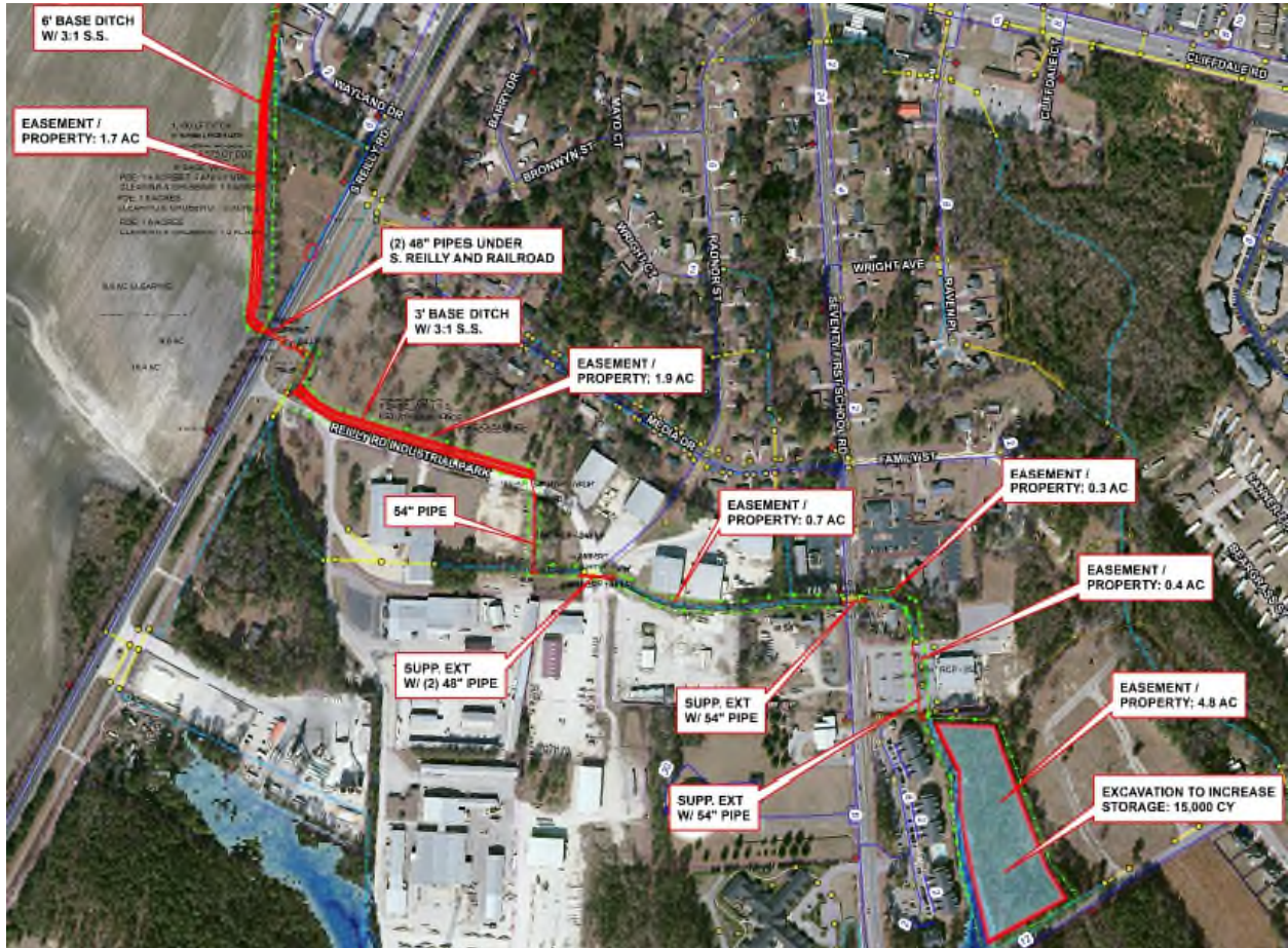
Figure 3 Option #3 proposes to grade a designated storage area in the vacant property north of Old Bounce Road
