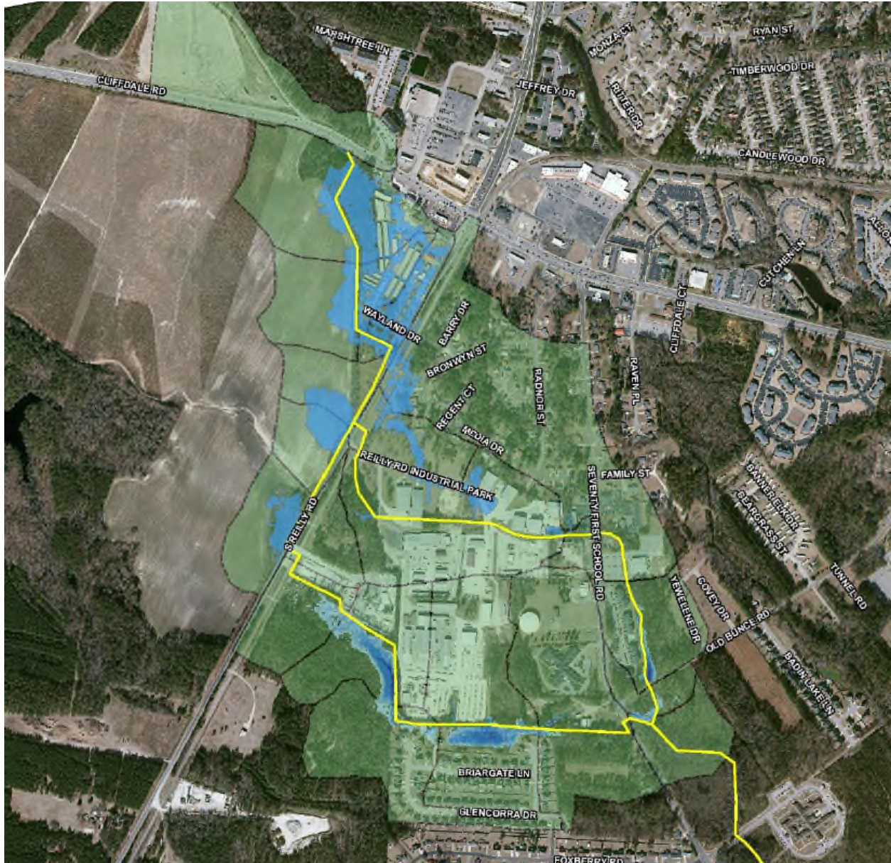
Figure 1 Modeling area used for drainage improvement assessment; existing condition 10-year storm flooding shown in blue, drainage area shown in green, and current drainage infrastructure is shown in yellow (on 2017 aerial basemap)
