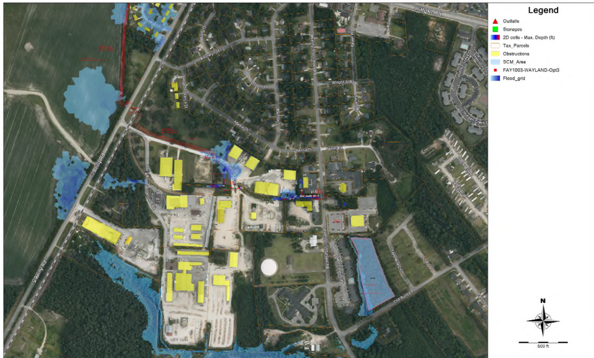
Figure 4 Results from H&H study showing inundation from 25-year storm event
