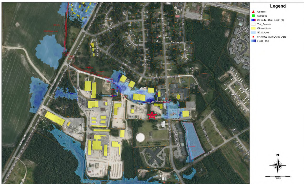
Figure 5 Results from H&H study - inundation from 100-year storm event. Red star indicates a Fire Station
