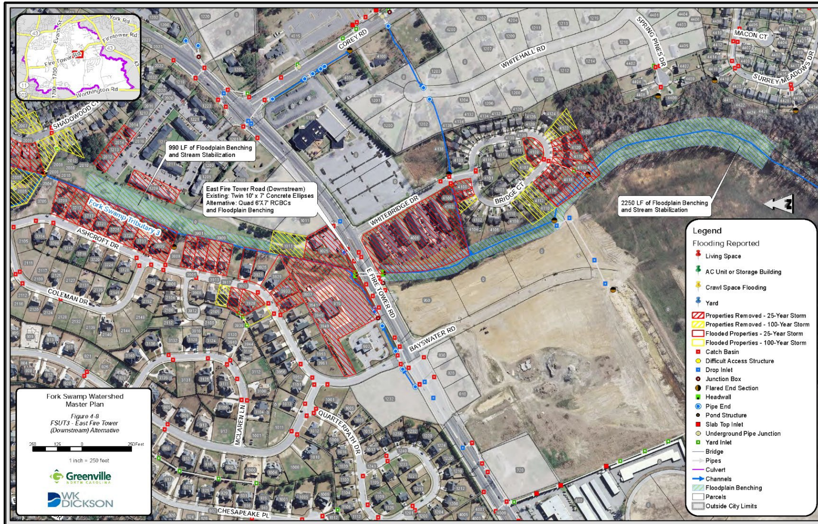
Figure 10. FSUT3 East Fire Tower Downstream Alternative
