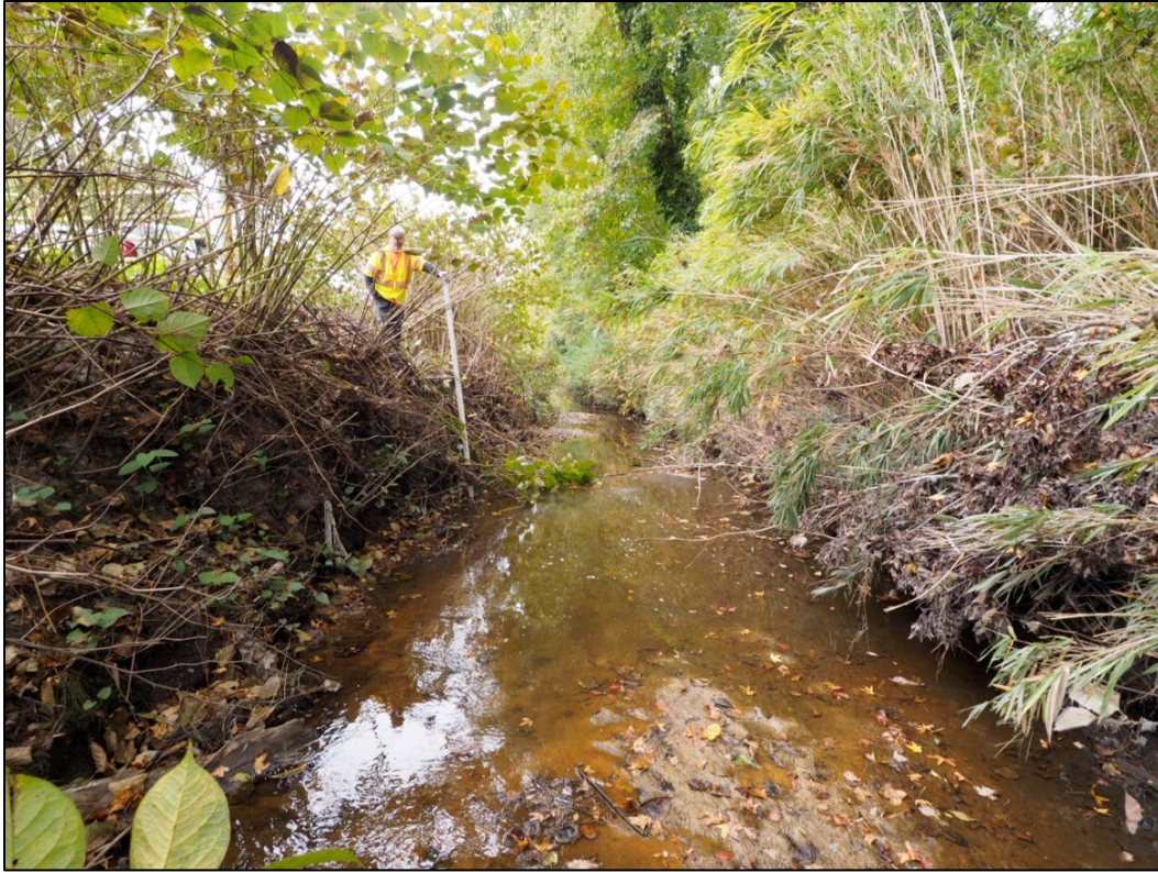
Figure 7. Fork Swamp Cross Section #1, Downstream of E. Fire Tower Rd. – 6 feet deep, 14 feet wide.
