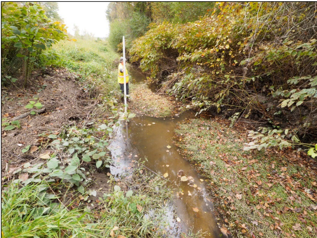
Figure 8. Fork Swamp Cross Section #2, Downstream of E. Fire Tower Rd. - 7 feet deep, 14 feet wide.
