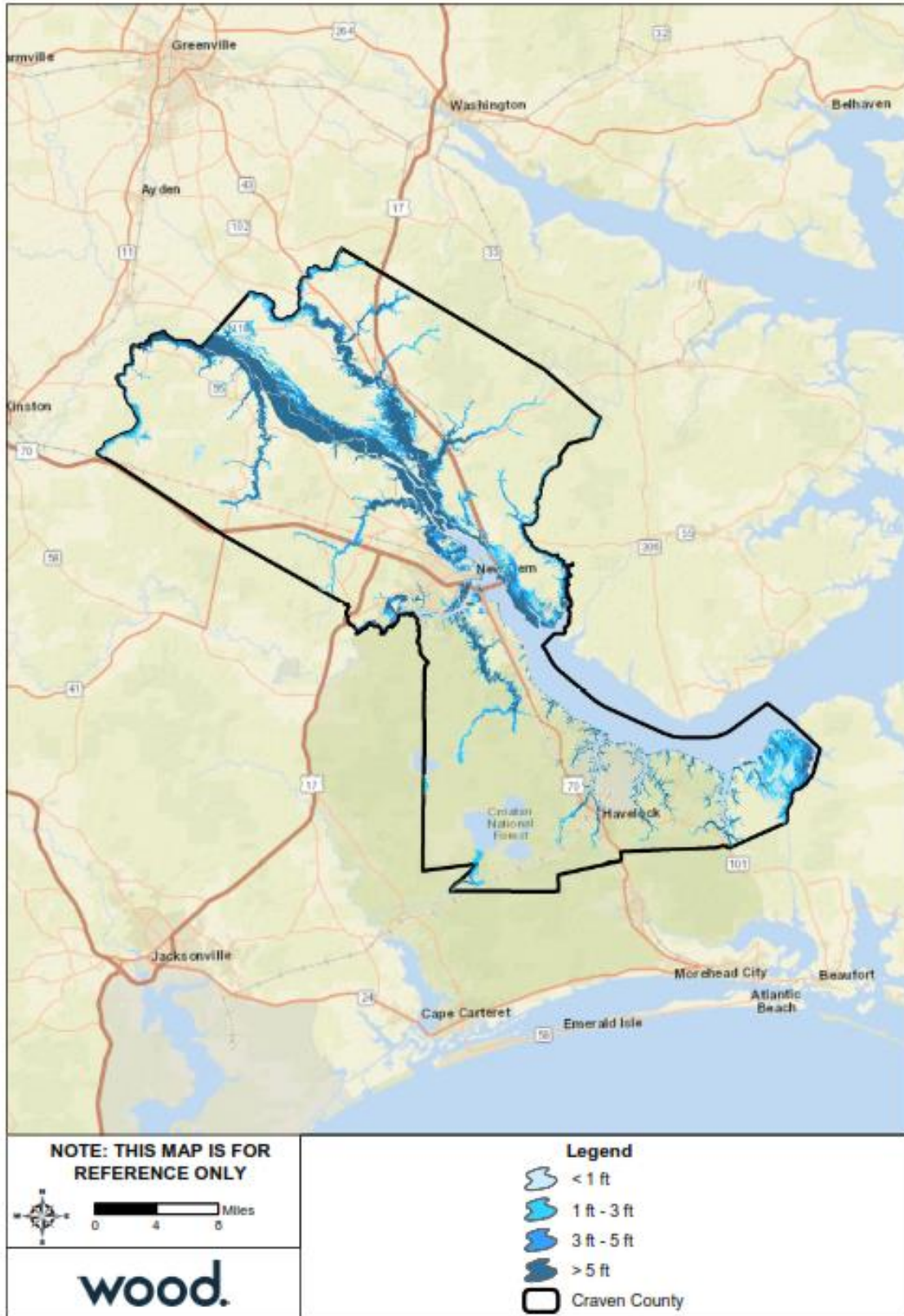
Figure C.22 – Flood Depth, 1%-Annual-Chance Floodplain, Unincorporated Craven County
