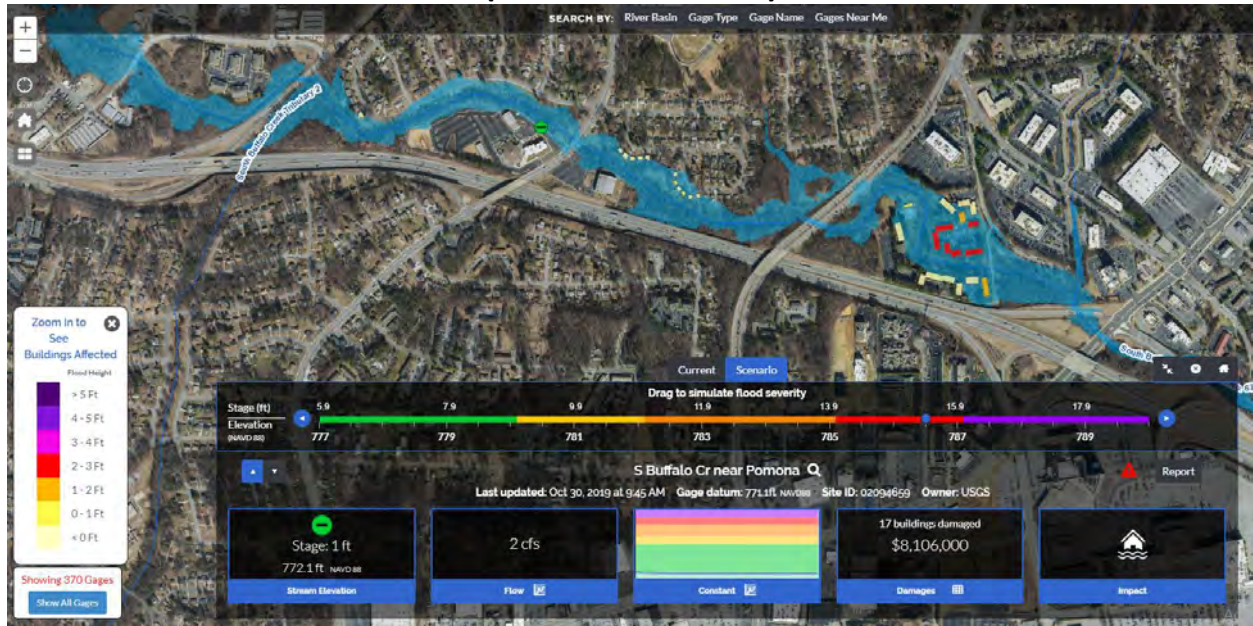
FIGURE 5.37: INUNDATION MAPPING AT THE SOUTH BUFFALO CREEK NEAR POMONA GAGE (STAGE LEVEL 15.4 FT)
